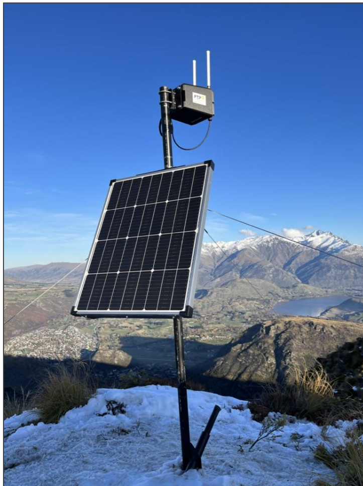
Figure 3 - Yarn Mesh Gateway deployed at around 1200m altitude, mounted on an Yarn Mesh Radio Comms Tower (RCT).
