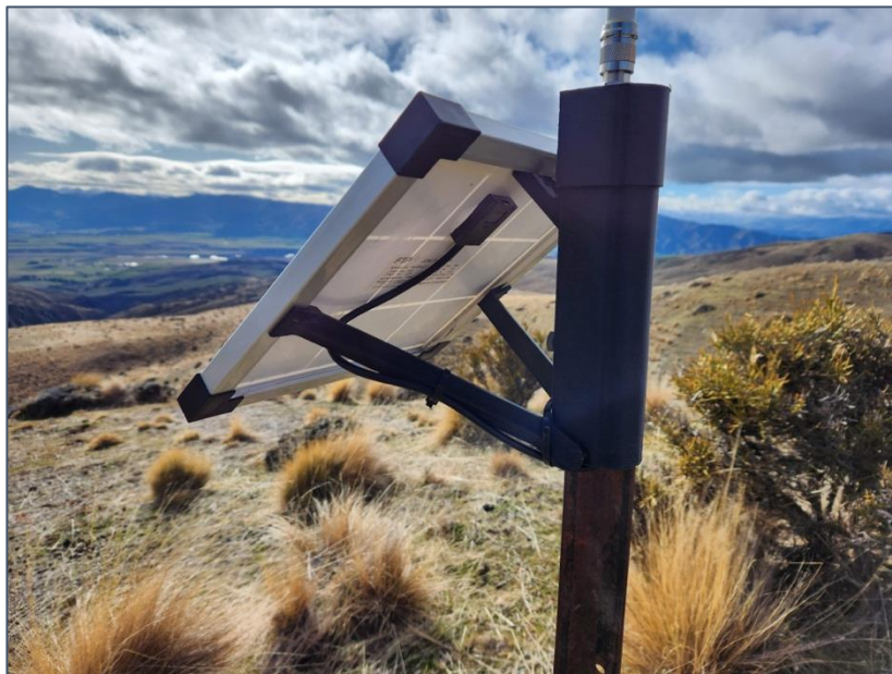
Figure 6 – Side view of the Yarn Mesh Relay enclosure, showing solar panel, solar panel mounting arms, main Relay enclosure body and RF antenna. Note: solar panel cable connection to Relay solar input plug.
